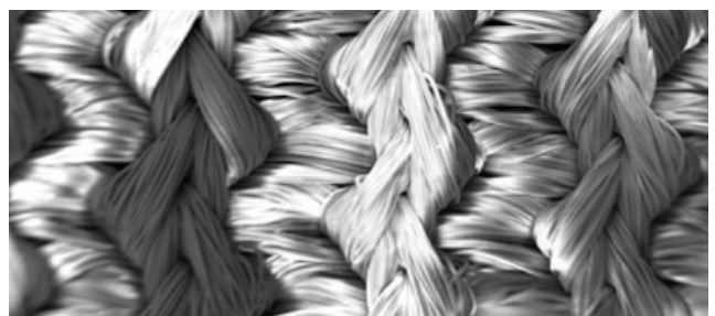
The patented knit structure that lets moisture out via micrometer pores
